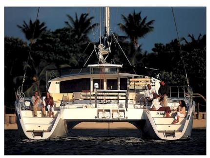
Catamarans these days are getting even more beamy, offering even greater stability being half their length or even greater in the beam. Catamarans with this kind of beam width have a static stability rating of well over 65 knots. The mast would more than likely break, well before any capsize.
